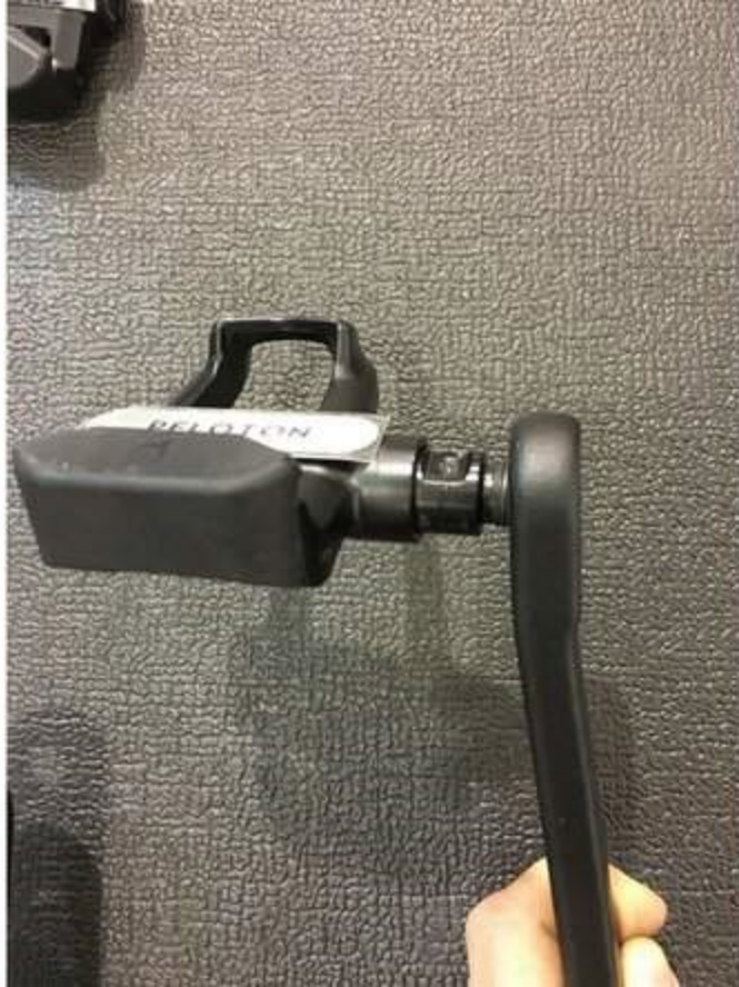
Failure Mode: Stripped crank arm threading.
