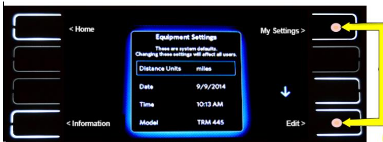
Accessing Hardware Validation mode: Simultaneously select the Right Side Upper and Lower menu softkeys.
