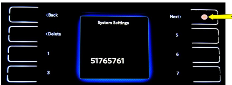
Enter Service Access Mode: Use number softkeys to type in Access Code > select Next
